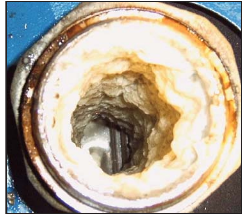
Figure 3: The inlet pipe of a new refrigeration dryer without prefiltration. Within one month, an emulsion of condensed water and compressor oil formed a mayonnaise-like deposit known as "white sludge" and the air flow through the dryer was excessively restricted.
